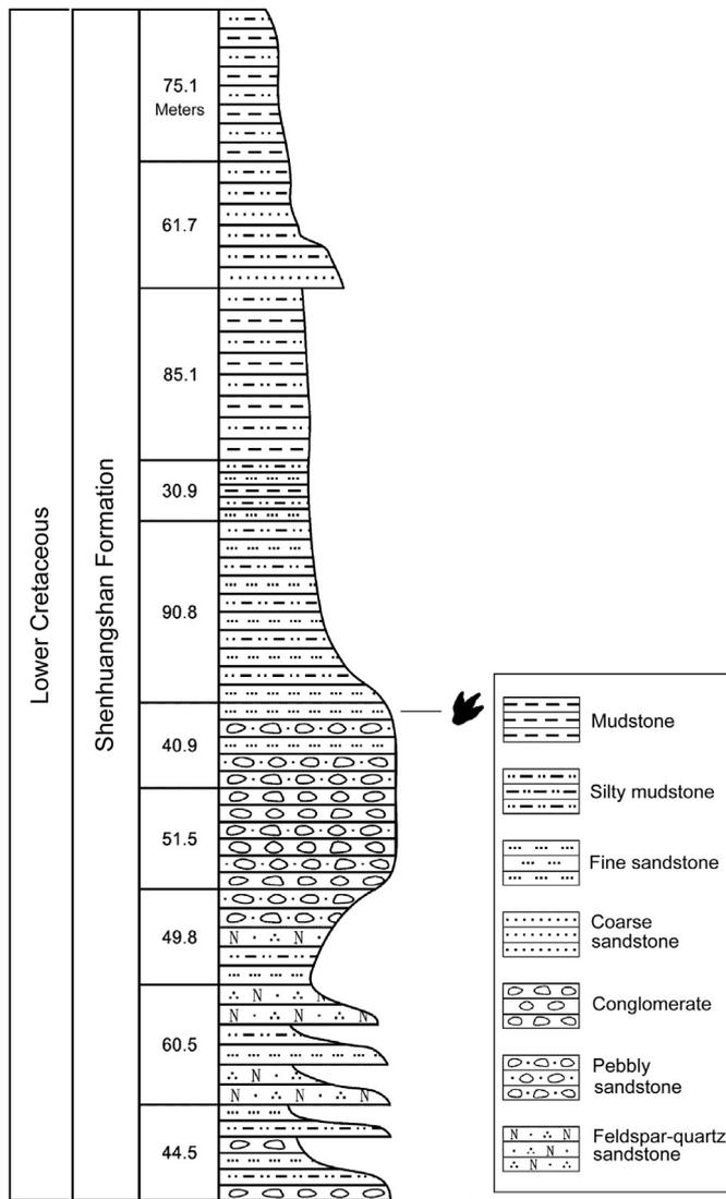
Fig. 2. Stratigraphic section of the Lower Cretaceous sedimentary sequences in the Jiuquwan area with the position of the footprint level.
